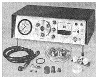
up to and including six standard microscope slides. Needle valves permit fine control of fluid entering or leaving chamber. Maximum temperature and pressure automatically controlled by internal electronics system.
