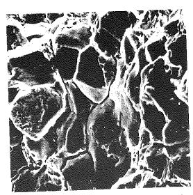
Closeup of area A shows intergranular cracking due to hydrogen embrittlement caused by improper bakeout after plating. 1600X
