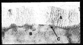
TEM thin-section of anodized Al surface, made specifically to reveal the thickness of the anodized layer, its structure and morphology, and to gain some insight into its uniformity. From TEM results, the image thickness is measured to be about 2000 Å. Arrows denote (A) Anodized layer, (B) substrate aluminum, and (C) interface.
