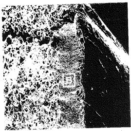
Fracture topography of plated steel component—area A failed in brittle fracture while area B failed in a ductile manner.
