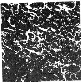
Closeup of area B showing dimple rupture of plating. Note spherical second phase particles located within some dimples. 2000X
