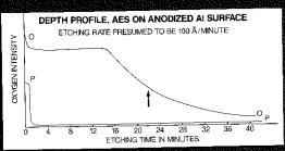
Auger electron spectroscopy (AES) depth profile into anodized aluminum layer using etching rate previously calibrated and presumed to be 100 Å/minute in Al<sub>2</sub>O<sub>3</sub>. The time for oxygen to drop to one-half its original intensity was 22 minutes, or an implied 2200 Å, which was in good agreement with the TEM results. Broad interface region can be clearly attrib-uted to surface roughness and variation in anodization thick-ness. P is confined to top 100 Å or less.
