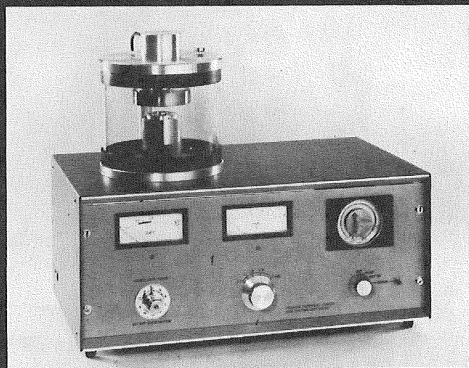
Diode sputtering system for scanning electron microscope specimens
