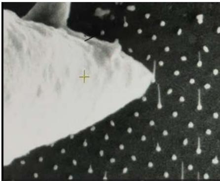
Figure 1. SEM image of vertically grown nanowire.
