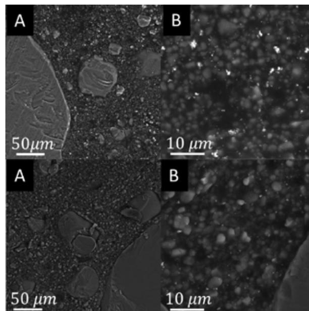
**Figure 1.** Representative backscattered electron SEM images of conventional mixed (top) and RAM (bottom) propellant formulations. A) and B) notation represent images taken with a primary magnification of 1000x and 6000x, respectively. Bright white spots in the B) images correspond to the Fe<sub>2</sub>O<sub>3</sub> catalyst particles.
