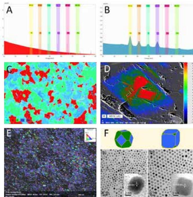
**Figure 1.** Analytical benefits of the Dual Excitation approach. A) Electron beam excitation; B) X-ray beam excitation; C) MicroXRF elemental mapping; D) Wavelength dispersive mapping; E) Platinum Nickel nanocrystals; F) Bright and dark field-like imaging.
