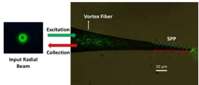
**Figure 1:** Optical image of the side emission from the tip apex of a gold coated tapered vortex fiber showing excitation and collection of radial beam using the SPP.
