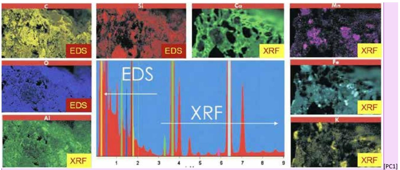
Figure 2. Example of Combo analysis using X-ray and e-beam excitation.
