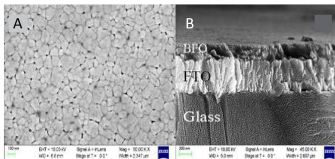
**Figure 1.** SEM images of the A) surface and B) the cross-section micrograph of the  $\text{BiFeO}_3$  thin film.
