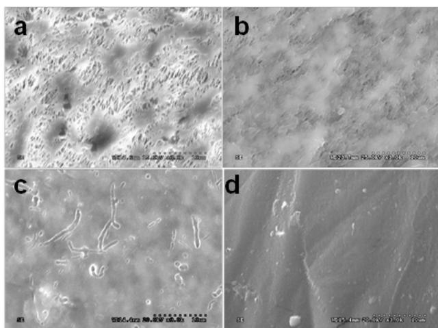
**Figure 1.** Different guanidium-based AEMs: a) Porous PTFE substrate; b) Partially penetrated composite membrane, AGM1, using 15% AEE-based polymer solution; c) Fully impregnated and crosslinked membrane, HGMC, using 7.5% HMDA-based polymer solution, and d) Fully impregnated and crosslinked.
