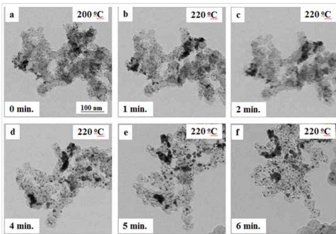
**Figure 1.** Video *in-situ* sequence images representing the degradation of a Pt/GC electrocatalyst of a fuel cell.
