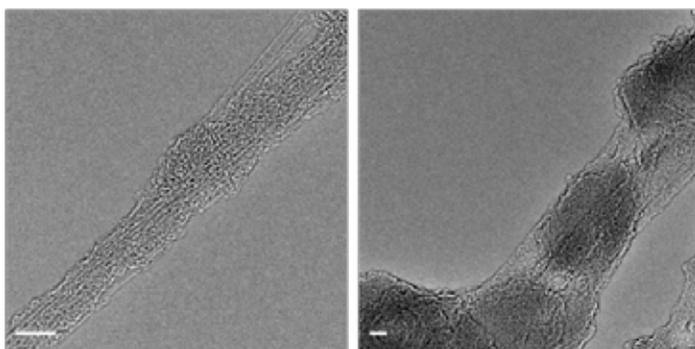
**Figure 1.** TEM images of GNTs (a) and PAA-wrapped GNTs (b). The scale bar is 10 nm.
