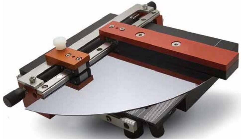
FlipScribe™ is a compact, stable, accurate, fast and low cost scribing and cleaving solution suitable for any lab; no utilities required. It provides a more accurate method for scribing than can be achieved with hand held tools, by integrating a robust diamond scribe into a sample platform with a fence guide design. Time required to align and scribe is about a minute.
