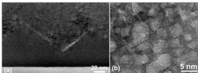
**Figure 1.** (a) Cross-section TEM of the HfO<sub>2</sub> coating deposited using  $t_i = 200 \mu\text{s}$  and  $\langle S_d \rangle = 7.3 \text{Wcm}^{-2}$ ; (b) HRTEM of the interlayer in (a) showing the porous structure.
