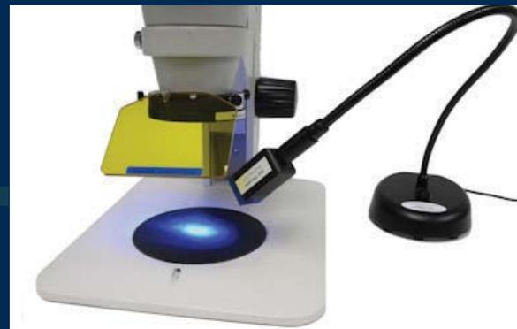
Adapt your existing lab stereo microscopes for fluorescence
