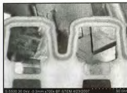
NAND double-gate cross-section in STEM
