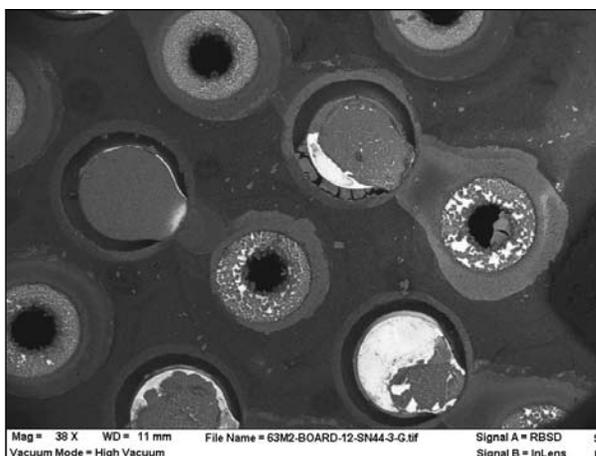
**Figure 1:** Low magnification image of contaminated pad on PWB. The bright areas contain gold and the dark areas on the pads contain nickel carbonate contamination. The contamination extends out onto the board surface.
