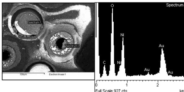
**Figure 2:** EDS data suggests the presence of C, O, and Ni on the gold plated surface.
