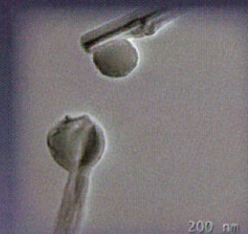
TEM image of the melted boron nanowire at bias of 30V
