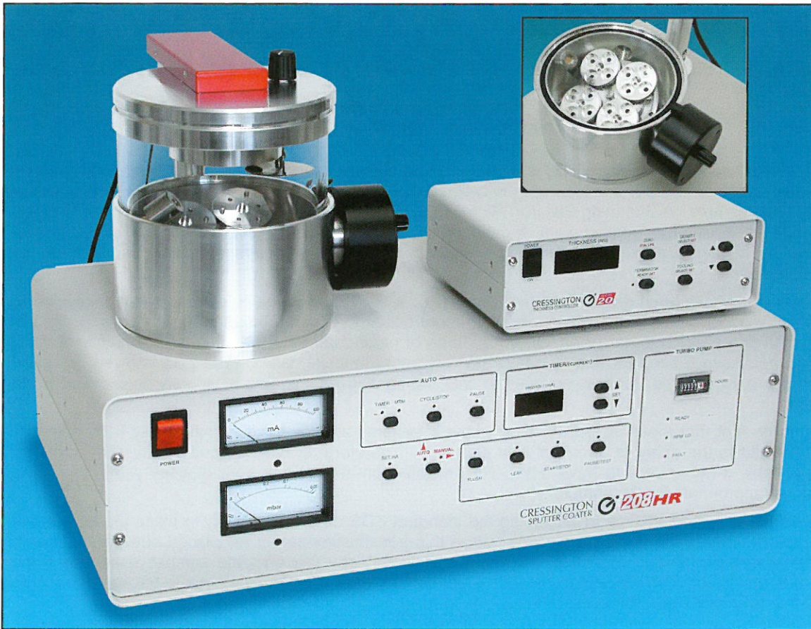
High Resolution Sputter Coater 208HR shown with Rotary-Planetary-Tilting Stage and Thickness Controller MTM-20 Fast coating with Turbo Vacuum for higher resolution requirements, such as FE-SEM
